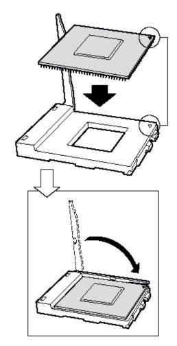
Figure 17: Inserting the Processor
